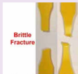
Figure 4: Brittle or ductile fractures can be distinguished visually.
