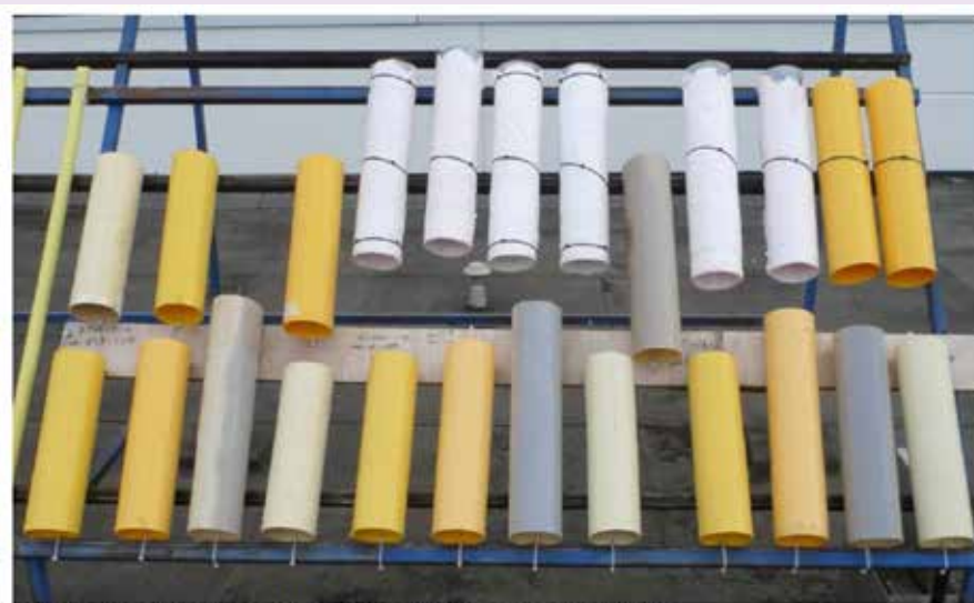
Figure 14: Overview of the pipes being exposed outside.
