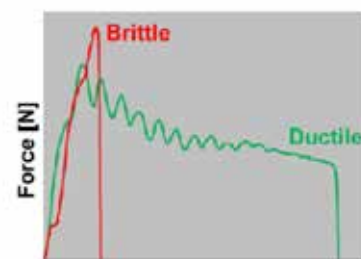
Figure 5: Different force-displacement graphs for brittle or ductile fractures.
