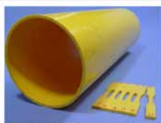
Figure 1: PVC-HI pipe with dumbbell-shaped specimens.
